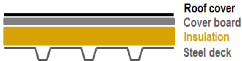
Figure 9 – Placement of cover board in a roof assembly (Image source: Rich Gallagher, Zurich)
